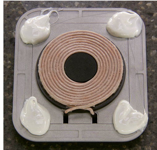
Figure D-2: 100% Silicone applied to transmitter
